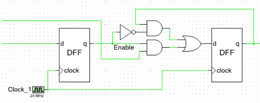
If access to a clock is needed, for example to generate a clock to send to a pin, then a 2x clock should be used to clock a toggle flip-flop. The output of that flip-flop can then be used with the associated timing analysis available.
