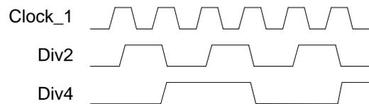
It may appear that the Div4 signal is generated by the falling edge of the Div2 signal. This is not the case. The Div4 signal is generated on the first Clock\_1 rising edge following a rising edge on Div2.
