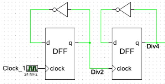
The report file indicates that one global clock has been used and that the single routed clock has been transformed using the global clock as the effective clock.
